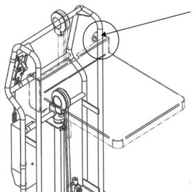
Lubricate spray grease between roller and shaft. (Every 3 months)
