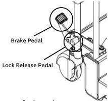
Brake (Wheel Lock) is equipped at right side caster. (Both wheels get locked at same time firmly)
