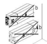
Charge the battery as per below diagram condition. Charging time is about 8 hours.
